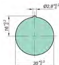
Pushbutton actuator SPO 01/ Front element of signal lamp SPO 02/ Pushbutton, signal lamp and potentiometer mounting
